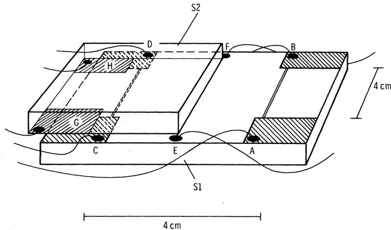
FIG. 1. Schematic representation of the apparatus. Bolometers:  $AB$  and  $CD$ . Resistance wire heater:  $EF$ . Capacitors:  $G$  and  $H$ . Substrates:  $S1$  and  $S2$ .
